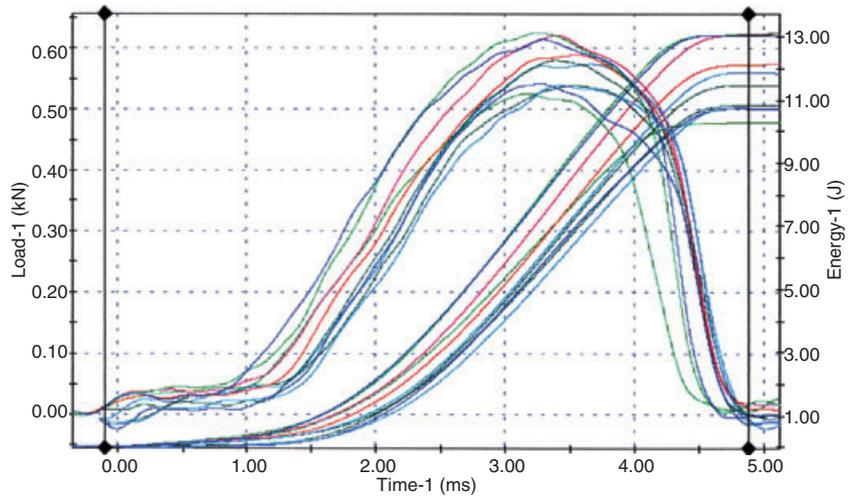
Fig. 2. Impact test results at 20 mph for 10 Pro-form™ specimens that had been conditioned for 1 h in artificial saliva at 37°C and then tested at 37°C.
