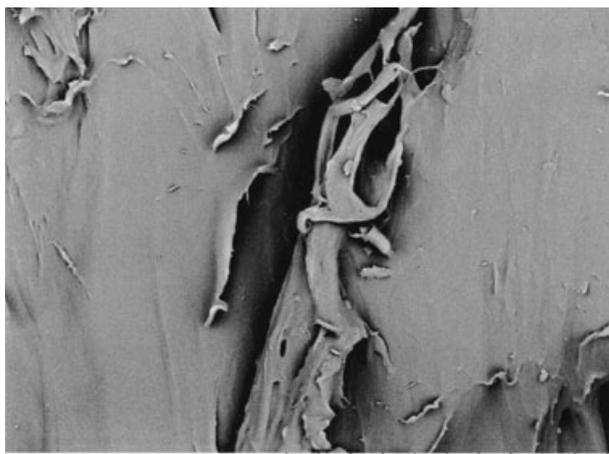
Fig. 5. SEM image near impact site of Pro-form<sup>TM</sup> sample after conditioning 1 h at 37°C in deionized water and loading at 20 mph and 37°C ( $\times 1000$  original magnification and scale bar length = 100  $\mu\text{m}$ ).
