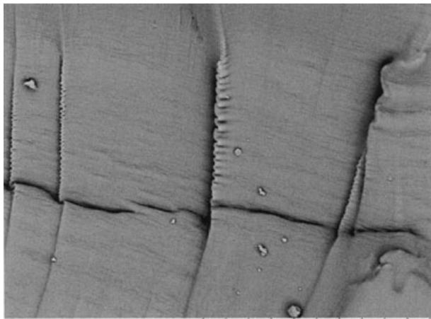
Fig. 4. SEM image near impact site of EVA sample after conditioning 1 h at 37°C in dry environment and loading at 20 mph and 37°C ( $\times 1000$  original magnification and scale bar length = 100  $\mu\text{m}$ ).
