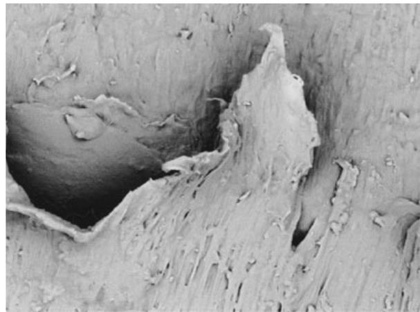
Fig. 6. SEM image near impact site of PolyShok<sup>TM</sup> sample after conditioning 1 h at 37°C in artificial saliva and loading at 20 mph and 37°C ( $\times 1000$  original magnification and scale bar length = 100  $\mu\text{m}$ ).
